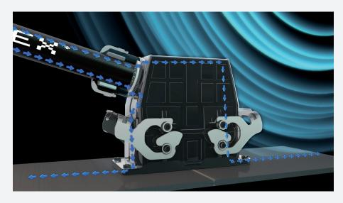
With cable glands, the maximum shielding performance can be achieved in designs that integrate the gland into the connector housing. These designs not only have beneficial shielding implications, they also eliminate a potential leak path between the connector housing and the strain relief, which increases the ability of the connector assembly to tolerate harsh operating conditions.
